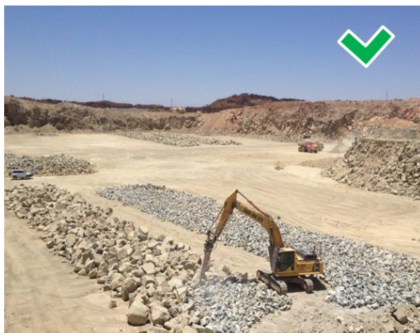
Figure 2: Recommended boulder hammering procedure.
