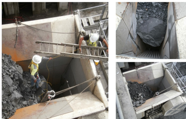
Figure 3: Secondary blasting inside a crusher to remove boulder blockage
