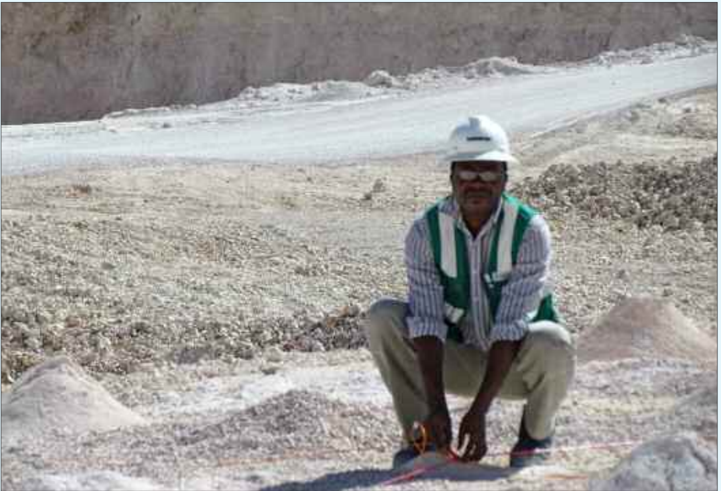
Figure 5. Connecting a 17ms Nonel connector to a surface trunk line at the limestone quarry.
