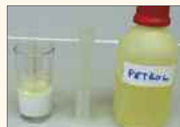
Fig.2 Disintegration and partial dissolution of explosive in petrol.
