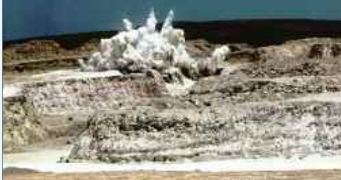
Figure 1. Blasting under ideal conditions without production of oxides of nitrogen in Majan limestone quarry.
