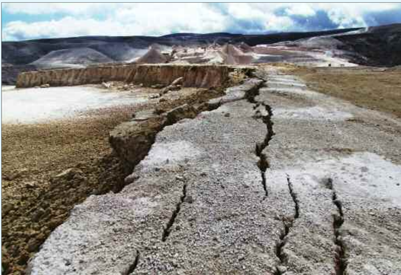
Figure 7. Back break as observed after bench blasting in Majan limestone quarry.
