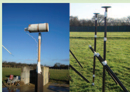
Figure 6. Mounted explosive charge and blast gauges.
