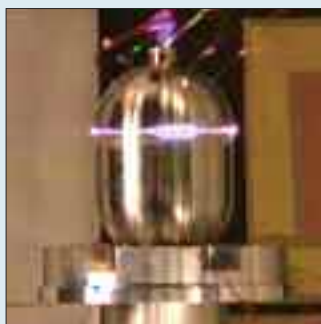
4b. Detonation products breach case, frame at +12 \mu s.
