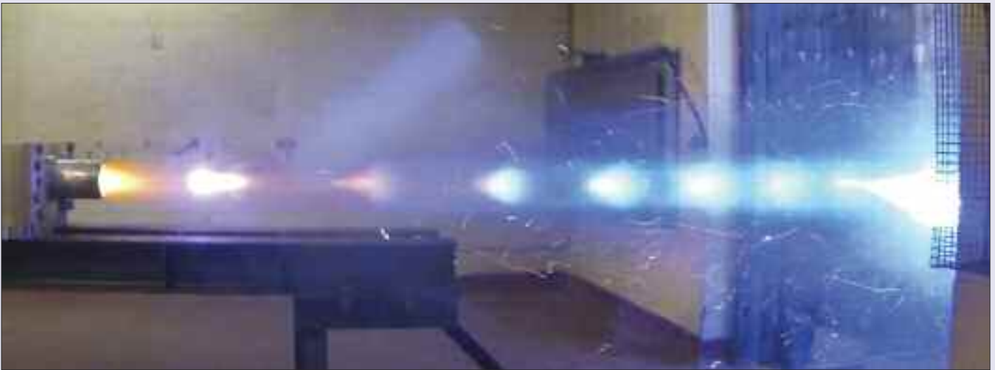
5-inch motor firing.
