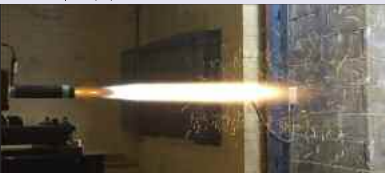
2-inch rocket motor with double cone and cylinder charge design.
