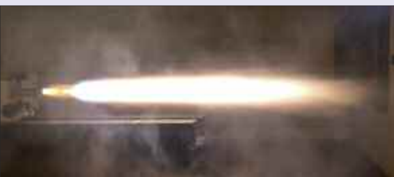
2-inch slotted radial motor firing.
