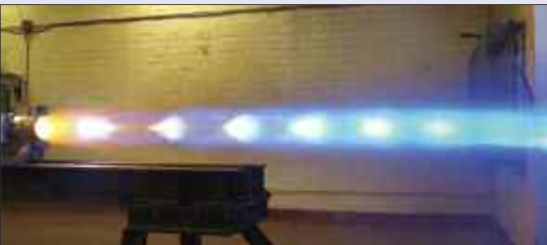
Firing of a 5-inch diameter rocket motor using 14 batches of RA mixed composite propellant.
