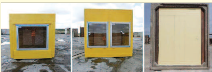
Figure 1. Typical glazing targets mounted in a single aperture cubicle and a double aperture cubicle, and a typical wall target mounted in a reinforced concrete cubicle (courtesy of DNV GL).
